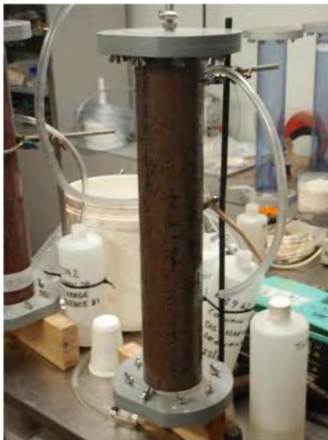
Figure A2.3: Photograph of Saturated Column
