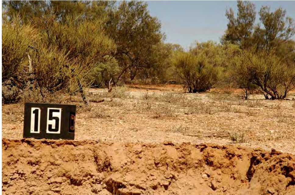
Plate 8: Calcrete rises are characterised by a surface lag of weathered calcrete overlying a stony loam, fine sandy (Lfsy) overlying a carbonate rubble in an Lfsy matrix. Platy, strongly laminated calcrete occurs, at this location, at 0.45 m below ground level.
